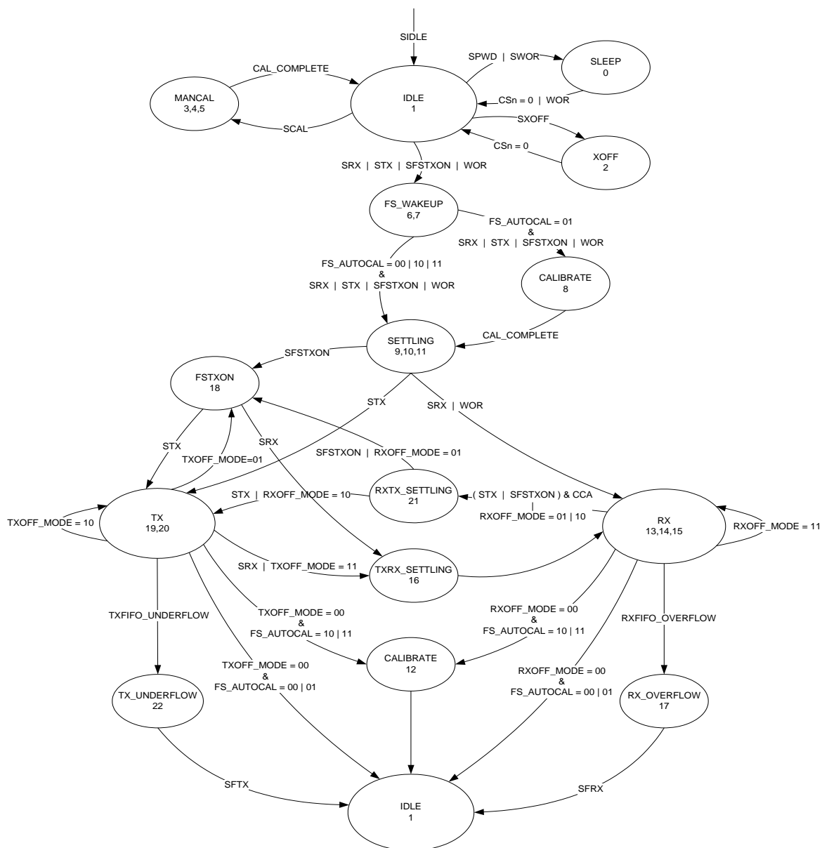
Figure 25: Complete Radio Control State Diagram
